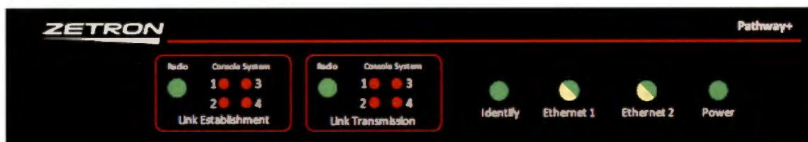
Figure 14. Front View of the Zetron Pathway+ Gateway
